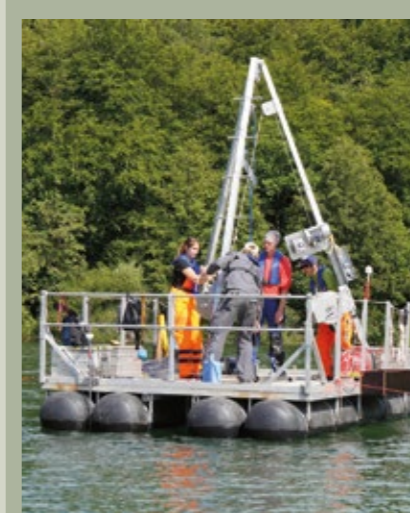
Fig. 2: The drilling platform floats on the Holzmaar and the scientists are ready to recover sediment cores from a water depth of 20 m.
